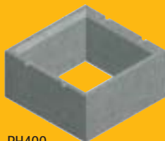
PH400 postiplokk 400 x 400 x 200 mm kulu 5 kpl/m mass 26 kg betoonikulu 110 l/jm
